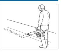
wide open throttle for at least 5 minutes every hour, and inspect/clean the spark arrester screen after approximately 40 hours of operation.
