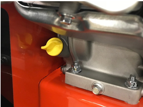
Figure 2.2, Left Side Oil Fill
