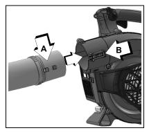
Do not assemble the opposite end of the curved blower pipe to the fan case.
