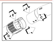
Note: Blower use will eventually loosen pipe connections. Exclusive positive locking system allows pipes to be tightened. If loosening occurs, remove straight pipe, and reinstall according to instructions 3 and 4.
