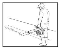
wide open throttle for at least 5 minutes every hour, and inspect/clean the spark arrester screen after approximately 40 hours of operation.
